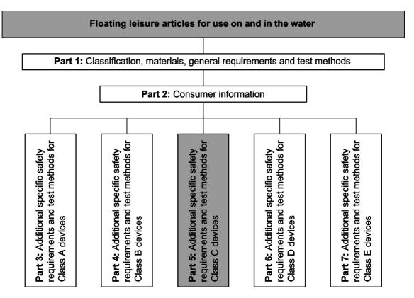
Compliance of a product to this standard requires that the requirements of the relevant specific part and, additionally, the requirements of EN 15649-1 and EN 15649-2 have to be met. If a product includes multiple use related to several classes, it has to meet the requirements of all these classes.
